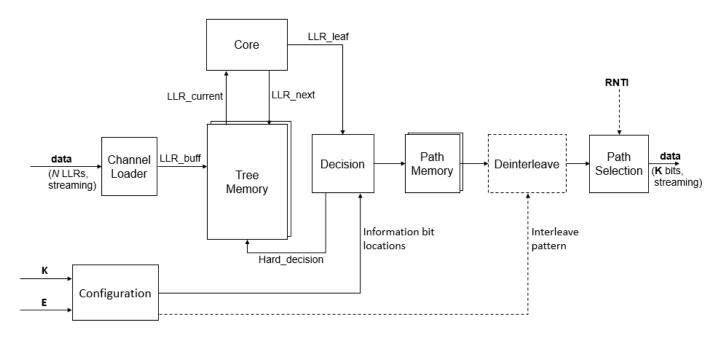
The block uses the Configuration stage when the  ${\bf K}$  and  ${\bf E}$  input port values change. The block computes the locations of the information bits and passes them to the Decision stage. Because the mapping patterns are computed as needed, rather than stored in hardware, the block supports all  ${\bf K}$  and  ${\bf E}$  values within the supported range. The Configuration stage also computes the interleave pattern when you set the **Link direction** parameter to Downlink.
