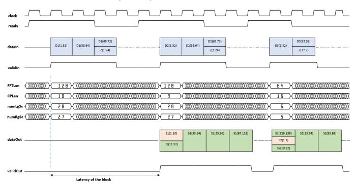
In the figure, D1 and D2 indicate the active data subcarriers, Z indicates padded zeros, and S1 and S2 indicate modulated output data symbols.
