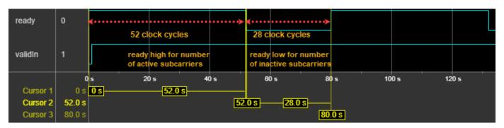
This figure shows the ready signal generation for the default block configuration (**FFT length** = 64, **Cyclic prefix length** = 16, **Number of left guard subcarriers** = 6, **Number of right guard subcarriers** = 5 and **Insert DC Null** = on) with a four-element column vector input.
