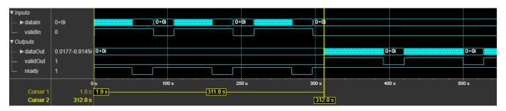
This figure shows a sample output and latency of the block when you specify a scalar input and set the **OFDM parameters source** parameter to **Input port**. For this example, **FFTLen** is set to 64, **CPLen** is set to 16, **Insert DC null status** is set to on, **numLgSc** and **numRgSc** are set to 6 and 5, respectively, and **Maximum FFT length** is set to 128.
