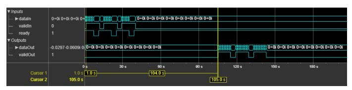
This figure shows a sample output and latency of the OFDM Modulator block when you specify an eight-element column vector input and set the **OFDM parameters source** parameter to **Input** port. For this example, **FFTLen** is set to **64**, **CPLen** is set to **16**, **Insert DC null status** is set to **0n**, **numLgSc** and **numRgSc** are set to **6** and **5**, respectively, and **Maximum FFT length** is set to **128**.
