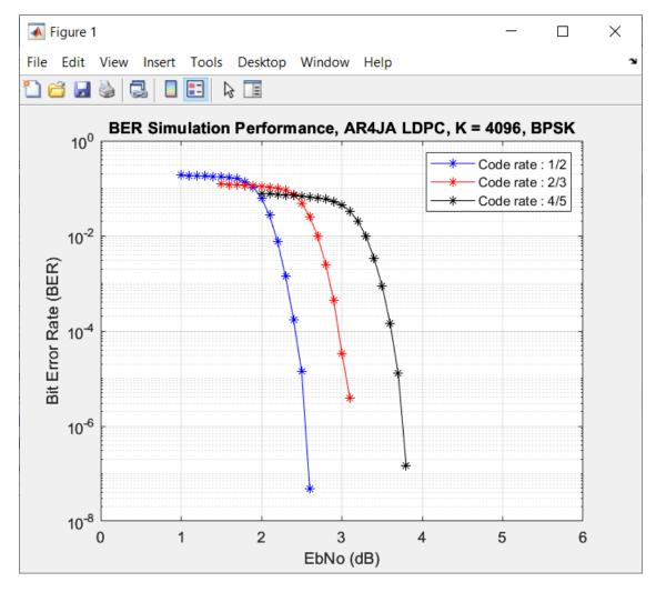
This plot shows the performance of the block for a 4 bit BPSK modulated LLR input for a block length of 16384 with code rates of 1/2, 2/3, and 4/5, respectively, when you set the **Configuration type** parameter to AR4JA LDPC.
