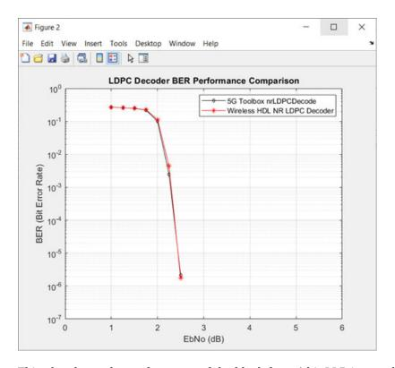
This plot shows the performance of the block for a 4-bit LLR input when you set the  $\bf Algorithm$  parameter to Normalized  ${\tt min-sum}$  .
