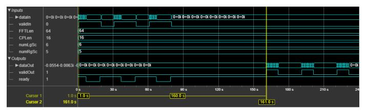
The block accepts input only when the **ready** signal is 1 (high). In this case, the block captures parameters on the first cycle when the input **valid** signal is 1 (high).
