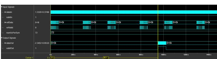
parameter is set to 72, and **numScPerSym** port is set to 72. The latency of the block is 951 clock cycles.
