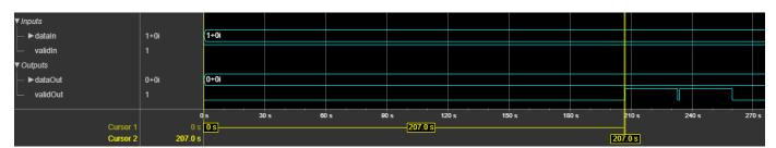
After calculation, the latency of the block is 207 clock cycles, as shown in the following figure.
