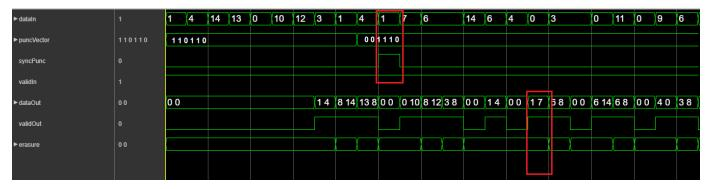
• Frame - You can only change **puncVector** at the start of a frame, indicated by **ctrl**. start. This waveform shows ufix4 input samples depunctured in Frame mode.
