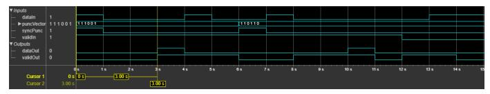
• Frame mode — When the puncture vector element is 1, the block stores the corresponding input data in a buffer. It waits till it encounters the next 1 in the puncture vector and then provides the previous buffered data as output.
