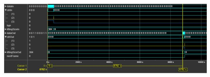
This figure shows a sample output of the NR LDPC Decoder block with latency. In this case, the **bgn**, **liftingSize**, and **numRows** input port values are set to 0, 384, and 4, respectively, and the **Number of iterations** parameter is set to 8. The latency of the block is 1,674 clock cycles.
