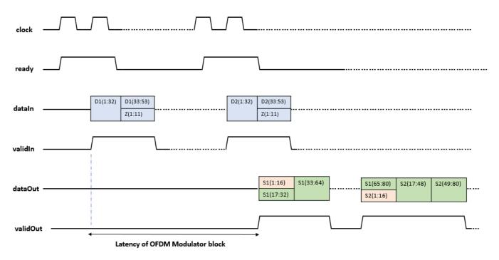
To provide 53 active data subcarriers of vector length 32, two cycles are needed. In this case, you must send the first set of data samples as D1(1:32), send the second set of data samples as D1(33:53), and pad the remaining samples with zeros Z(1:11) to make the complete vector. Similarly, the block processes D2 based on the block parameter values.
