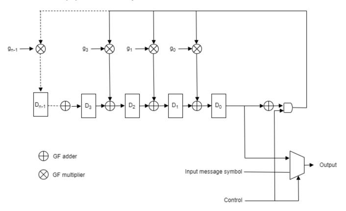
In this figure,  $g_0$ ,  $g_1$ ,  $g_2$   $g_3$ , and so on up to  $g_{n-1}$  represent the generator polynomial coefficients and  $D_0$ ,  $D_1$ ,  $D_2$ ,  $D_3$ , and so on up to  $D_{n-1}$  represent registers, where n is equal to 255 – k and k is the **Message length (k)** parameter value specified on the block mask. The registers store the parity symbols.
