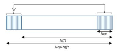
The LTE OFDM Modulator block uses FFT size of 2048 for all NDLRB resources to avoid multiple IFFTs. The block uses CP values corresponding to NDLRB 100.
