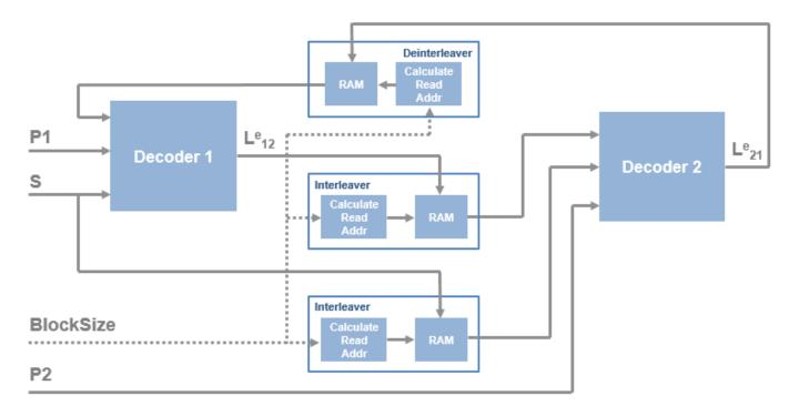
The odd half-iterations compute the likelihood ratio from uninterleaved bits (P1, S, and deinterleaved results of P2 decoding). The even half-iterations compute the likelihood ratio from the interleaved bits (P2 and interleaved results of P1 and S decoding).
