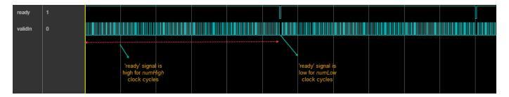
numHigh = (FFT length + CP length - 1) \* Maximum FFT length / FFT length + 1 = (128 + 10 - 1) \* 16 + 1 = 2193 clock cycles.
