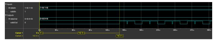
This figure shows a sample output and latency of the block when you specify a two-element column vector input and set the **OFDM parameters source** parameter to **Input port**. For this example, **FFTLen** is set to **64**, **CPLen** is set to **16**, **numLgSc** is set to **6**, **numRgSc** is set to **5**, and **Maximum FFT length** is set to **128**.
