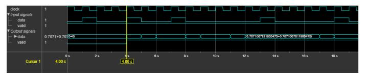
This figure shows a sample output when you select BPSK, QPSK, 16-QAM, 64-QAM, and 256-QAM modulations by using the **modSel** input port. The latency of the block varies with the modulation selection.
