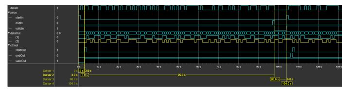
The latency of the block is three clock cycles, so the block returns the first encoded output data after three clock cycles. In the Terminated mode, after the end of the frame, the block resets the encoded states to all zeros state by appending (Constraint length – 1) bits. So, the waveform shows the frame gap of six (Constraint length – 1) clock cycles between the end of the frame (ctrlIn.endIn) and the start of the next frame ctrlIn.startIn.
