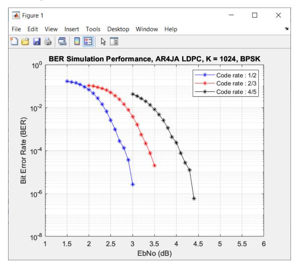
This plot shows the performance of the block for a 4 bit BPSK modulated LLR input for a block length of 4096 with code rates of 1/2, 2/3, and 4/5, respectively, when you set the **Configuration type** parameter to AR4JA LDPC.
