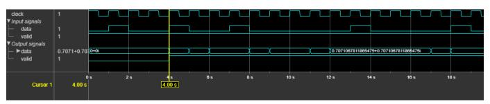
This figure shows a sample output when you select BPSK, QPSK, 16-QAM, 64-QAM, 256-QAM, and pi/2-BPSK modulations by using the **modSel** input port. The latency of the block varies with the modulation selection.
