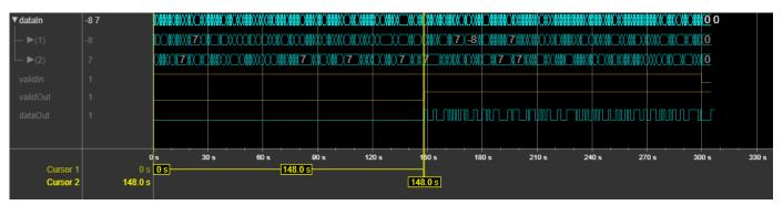
The second waveform shows three frames in terminated operation mode. The input is unsigned 4-bit samples, and the block is using the trellis (7,[171 133 112]). The **Traceback depth** is 32. The input and output **ctrl** buses are expanded to show their three control signals. The latency from each input **ctrl**.start to output **ctrl**.start is also 148 clock cycles.
