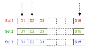
Output parity symbols D1D1D1D2D2D2D3D3D3 ----- D15D15D15
