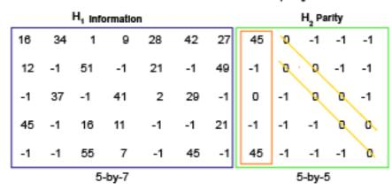
Mix of double-diagonal followed by a single-diagonal lower triangular — Contains a double-diagonal matrix with the extended rows and columns as a lower triangular part with 0s on the diagonals, and -1s in the rest of the parity part. These matrices are used in the 5G NR communication standard.
