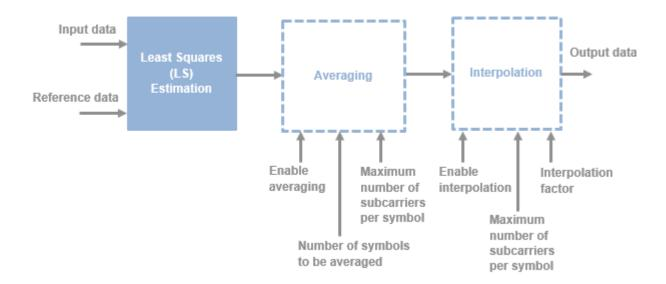
The Averaging block accepts the LS estimates and averages the corresponding subcarriers with valid LS estimates over the number of OFDM symbols to be averaged provided in the block mask. This figure shows a sample output of the OFDM Channel Estimator block when only averaging is enabled. In this case, the **Number of symbols to be averaged** parameter is set to 4, **Maximum number of subcarriers per symbol** parameter is set to 16, and the **numScPerSym** port is set to 4.
