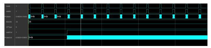
This figure shows the output data when you set the **Output data sample rate** parameter to Match output data sample rate to NDLRB parameter. For NDLRB value 25, the output sample rate is 7.68 MHz, and the block returns valid output data at every fourth cycle.
