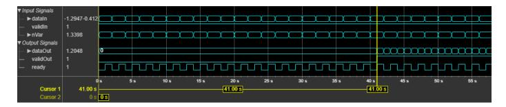
This figure shows a sample output and latency of the block for input data of type fixdt(1,16,14) when you set the **Modulation source** parameter to Input port, the **Decision type** parameter to Hard, and the **Output type** parameter to Vector, and specify the **modIdx** input port value as 3 (32-APSK). The latency of the block is 59 clock cycles.
